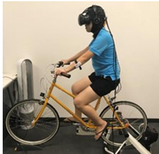
Figure 3: Instrumented bicycle used in the experiment
